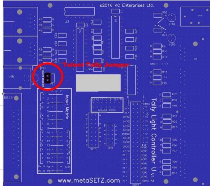
The jumper is located directly behind the USB connector. Short the two pins together with the included jumper to turn off all the talent tallies.
